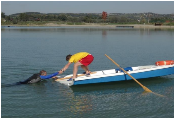
PHOTO 3. INNOVATIVE LIFEBOAT WITH AN OPEN STERN AND A WIDE DECK.
