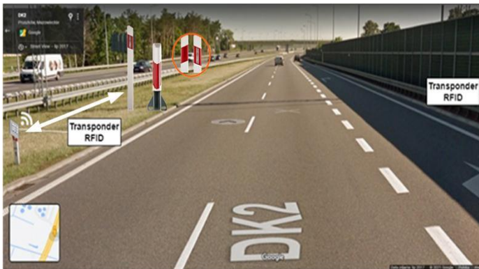
FIGURE 3 RFID TRANSPONDER IN ROAD INFRASTRUCTURE
